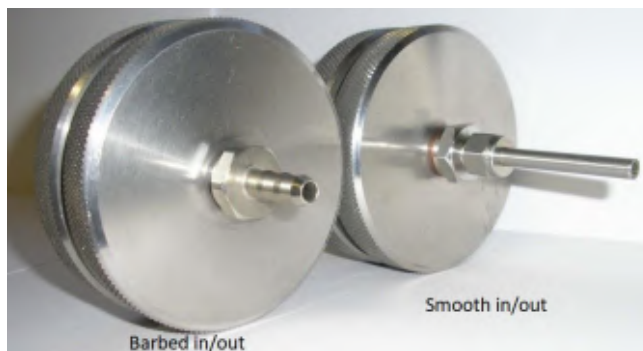
Triple flange with gas in/out nozzles
