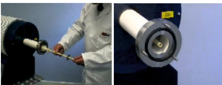
Insertion of the radiation shields in to the work tube
