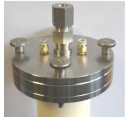
Triple flange end seal with thermocouple gland
