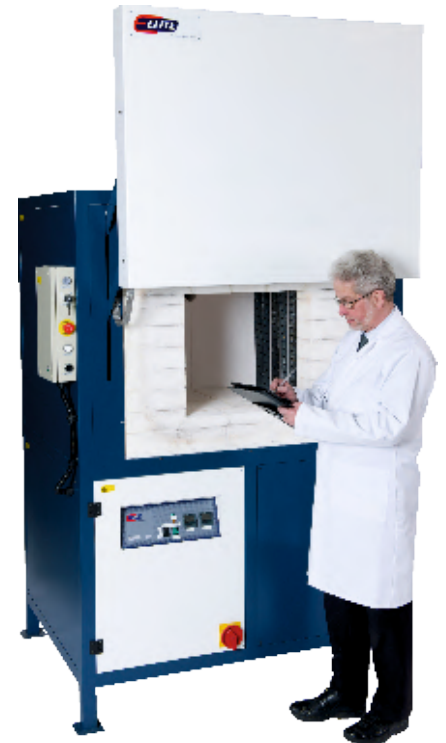
BRF16/35 with electrically operated door option
