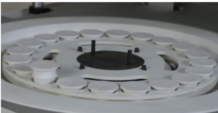
Weighing with crucible lids closed
